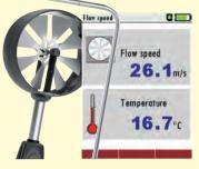
using vane probe or Pitot tube with flow rate calculation
