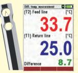
using thermocouples with 2 standard K-type sockets
