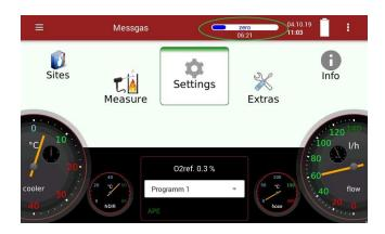
The remaining time until the Zero point measurement ends is displayed.
