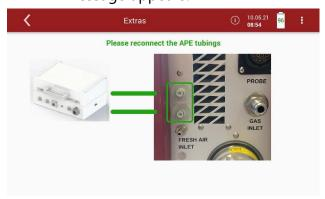
► Connect the Acid Dosing Unit APE to the analyserafter you have performed the leak test.
