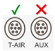
If an optional acid dosing unit APE is used, you can only use the connection T-AIR (T-air).
